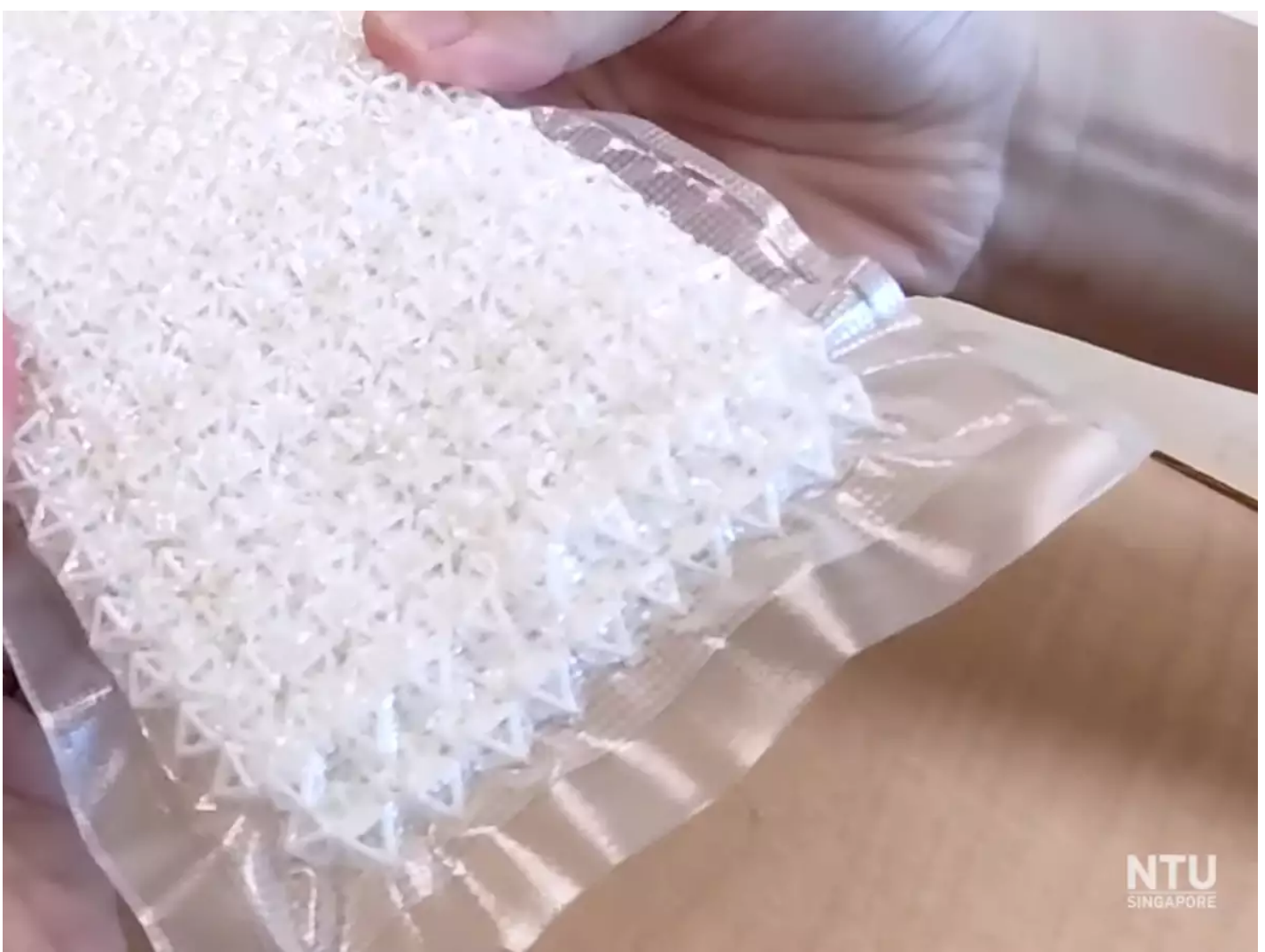
When the fabric is put inside a vacuum-packed plastic envelope, it stiffens up to reach its rigid state. NTU
